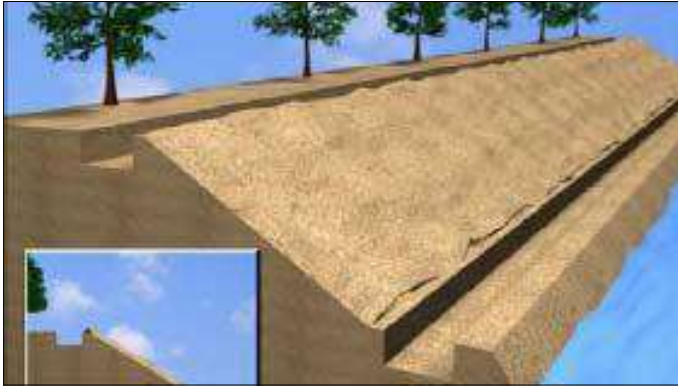
Dressing of the Embankment Slope
