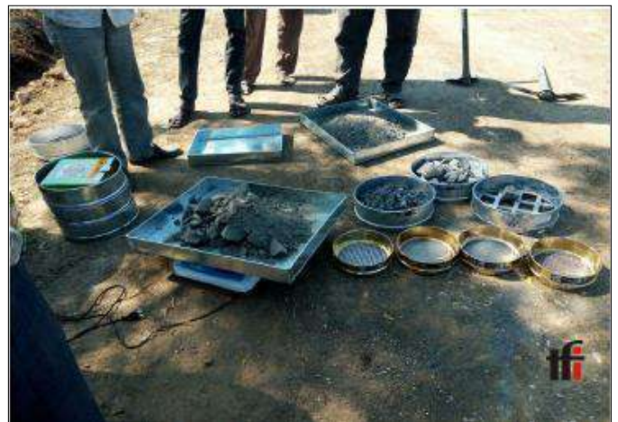
Gradation Test of GSB on site
