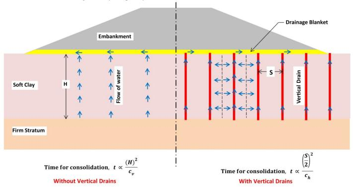
The use of vertical drains to accelerate consolidation of fine-grained soils has a history of almost 100 years starting with the introduction of sand drains in the 1920s and subsequent development of cardboard wick drains in the 1930s and 1940s. Large scale use of pre-fabricated vertical drains (PVDs) or band drains with a polymer core and a polymer geotextile filter jacket started in the 1980s.
